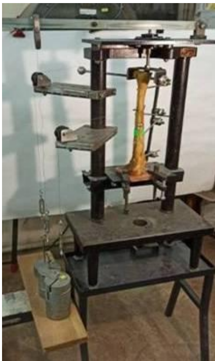
Testing equipment to study the reliability of fixation of bone fractures
