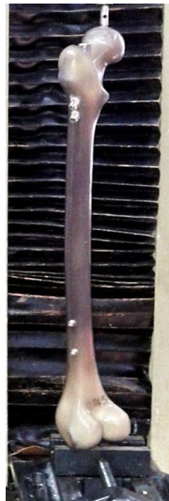
Synthetic models for studying the strength of the femurs
