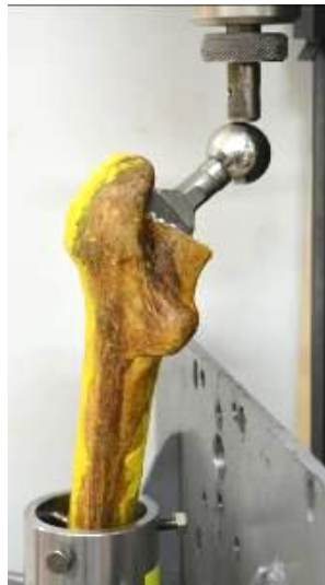
Investigation of the stiffness of the hip joint
