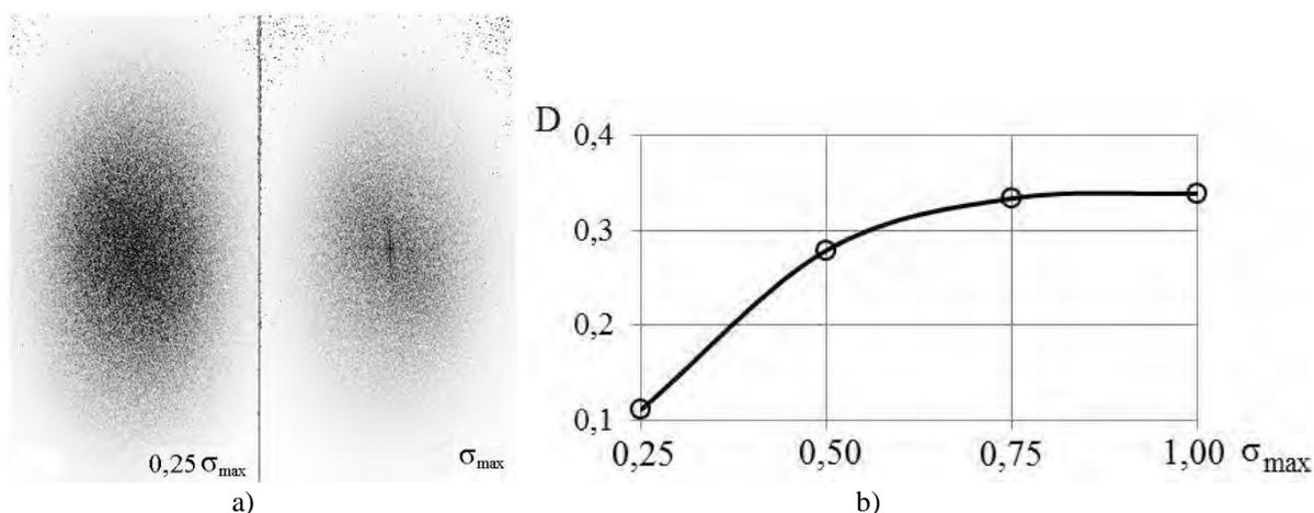
**Fig. 2 - Characterization of the deformation relief on the surface of the steel 45 specimen: a – the Fourier spectra of the surface after  $10^5$  loading cycles at the stress  $\sigma_{\max}$  and  $0.25\sigma_{\max}$ ; b – the kinetic behavior of the histogram for the speckle-pattern image of the deformation relief**
